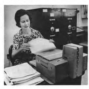
JOHNNIE JOHNSON (9000) demonstrates rapid process of reducing documents to microfilm with a portable automatic unit. The equipment is available by calling Section 7332-1. After microfilming, original documents are destroyed thus reducing need for bulky file cabinets.
